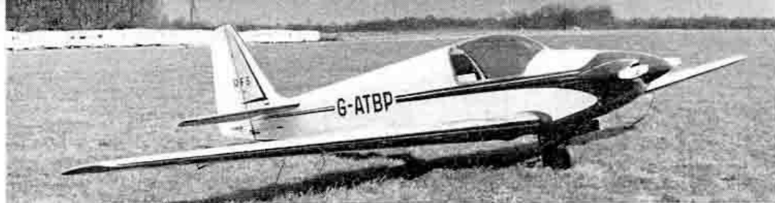
"The unconventional bicycle undercarriage arrangement, with a retractable mainwheel and wire outriggers with tiny plastic wheels attached, works surprisingly well" "Flight" photograph
